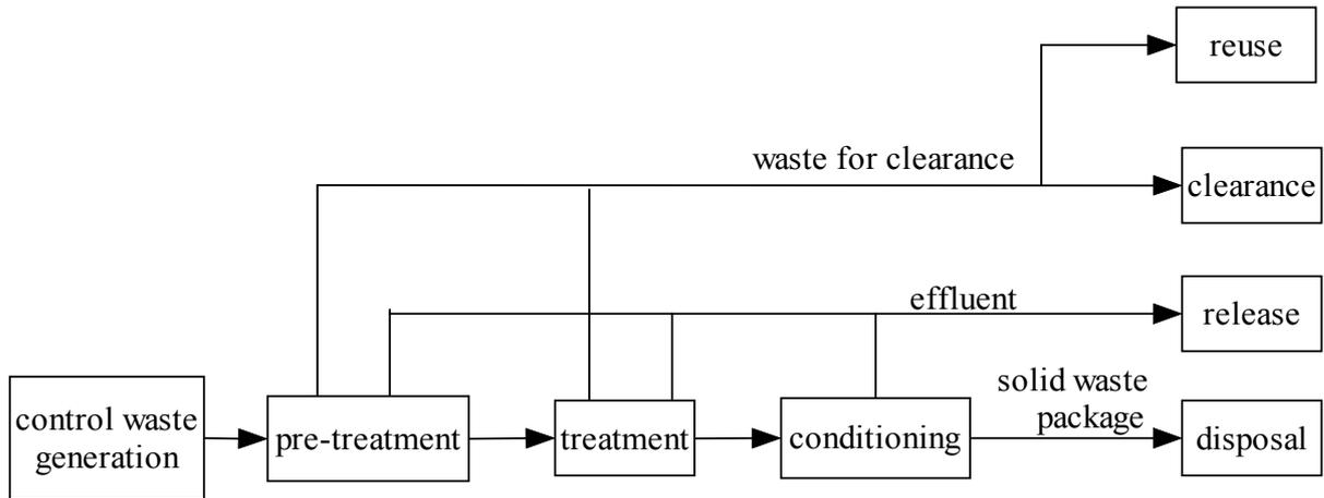
**Figure 4 Basic Steps towards Radioactive Waste Management**
