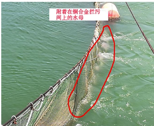
图4 附着在铜合金网上的水母 Fig.4 Jellyfish attached to a web of copper alloy
